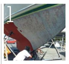
speed things along, Osmosis Solutions use a HotVac system where large blankets are attached to the hull and heated to temperatures exceeding 70°C, which exposes any weak areas and literally sucks all the remaining moisture from the hull, a great idea if you're eager to get back into the water.
